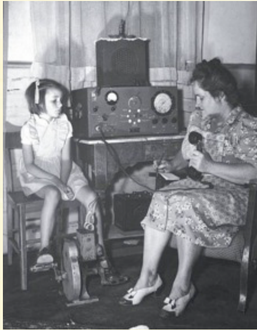
Traegar Pedal Radio Photo: Courtesy of the Royal Flying Doctor Service of Australia
